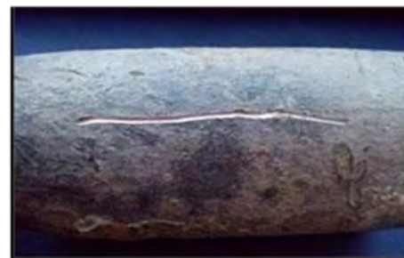
Picture of a Scratch on a Lead Service Line
