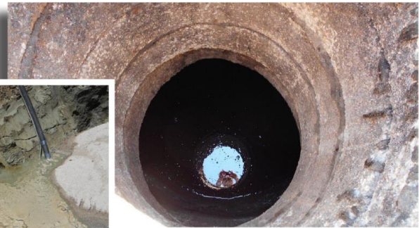
(Pictured left): Drilling a monitoring well on the site of an old refinery in Gordon; (right center): looking down at the reflection from free product floating on groundwater in an abandoned sewer in Lincoln's Telegraph District; (right bottom): sampling an abandoned sludge pit on the site of an old refinery in Gordon; (center): removing the floating product and contaminated groundwater from an excavation in Lincoln's Telegraph District.
