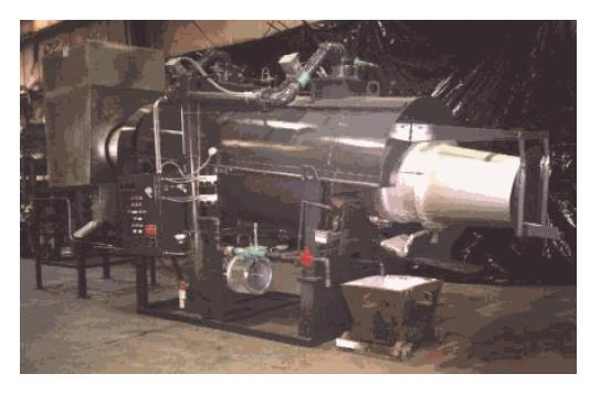
Figure 1: Photograph of Coreco Sweat Furnace and Afterburner (Models 1231 and 1848)
