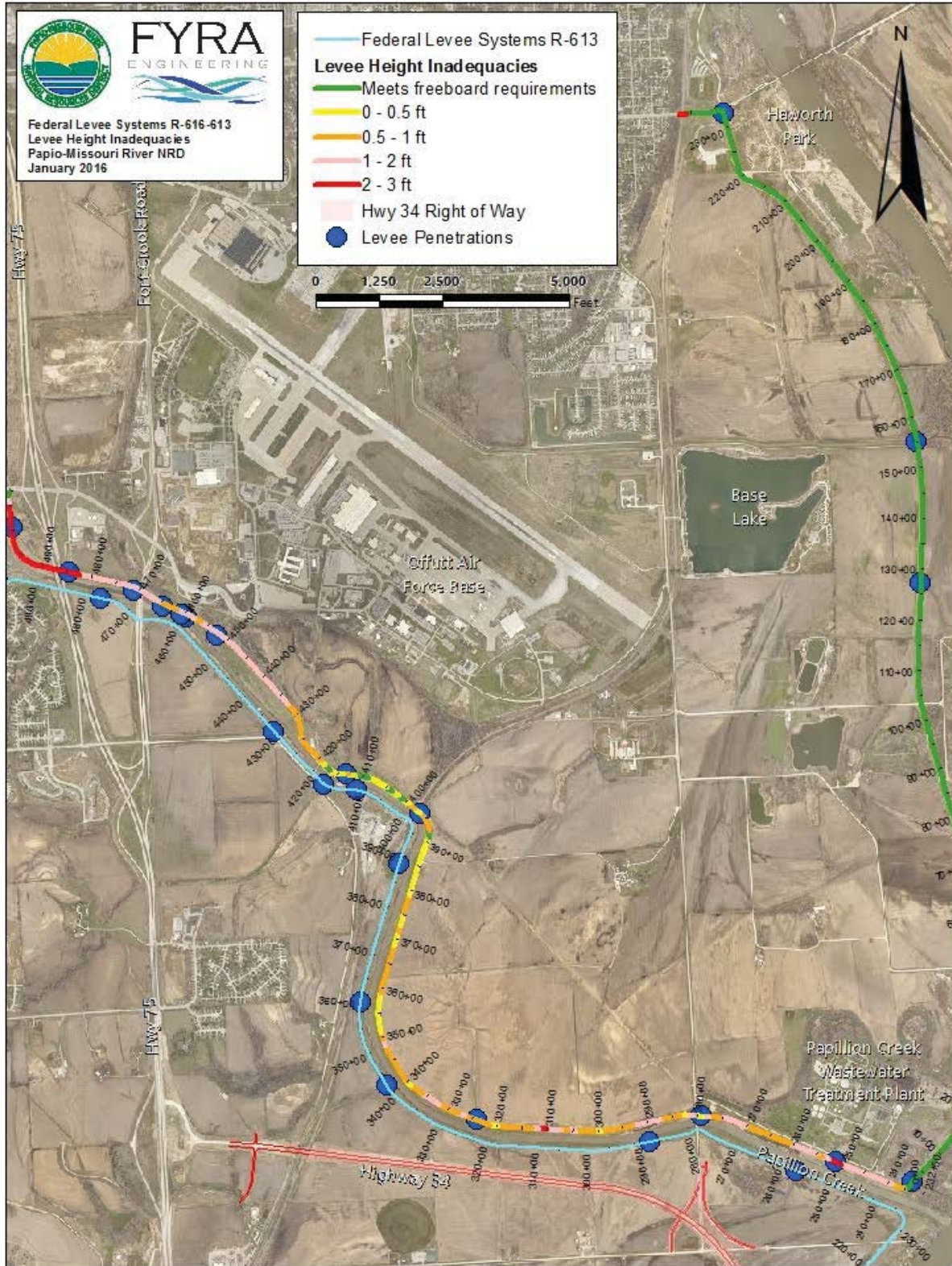
Figure 3 – R-616-613 AREAS WITH INADEQUATE FREEBOARD
