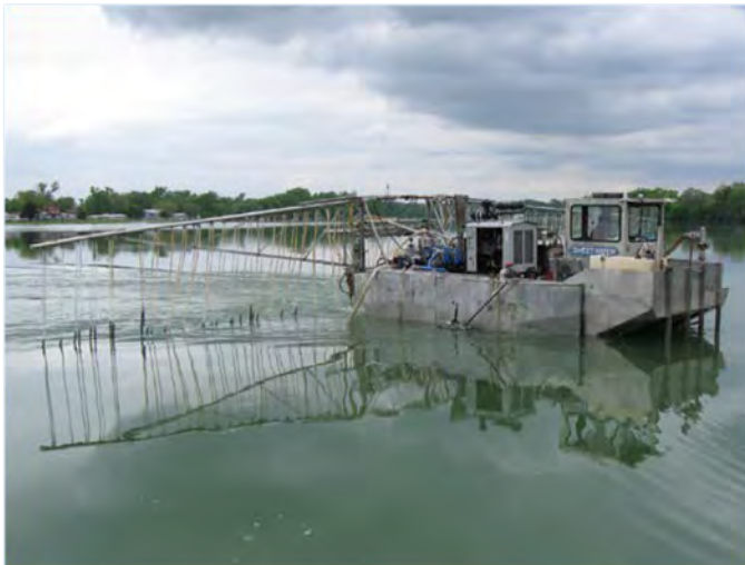
Application of alum and sodium aluminate to Carter Lake
