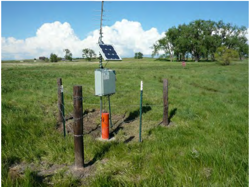
Water level monitoring well in Buffalo County. These wells, installed by the University of Nebraska-Lincoln, send water level measurements to Lincoln via telemetry. This type of well could be monitored for water quality as well.
