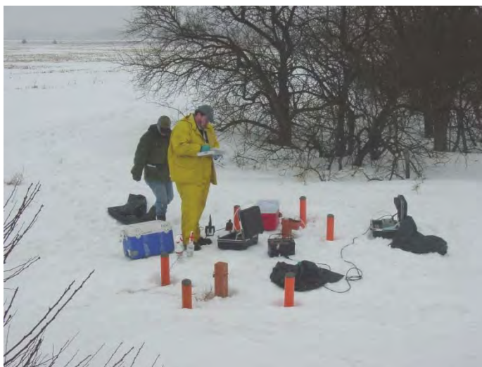
Contractors sampling monitoring wells in eastern Nebraska.
