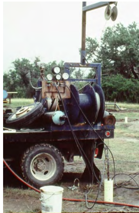
Mechanical Integrity Test at CBR
