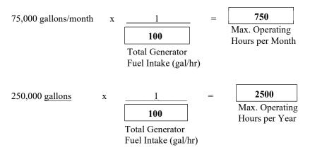
The maximum operating times are based on all of the generators at the facility. The total amount of time each generator is operated should be added together and not exceed the maximum operating times calculated. For example, if you have two generators, one is operated for 50 hours one month and the second is operated for 100 hours the same month, you are in compliance with this condition because your total operating hours (150) is less than 750.
